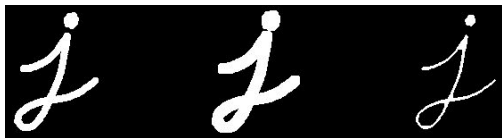
Left the original image. Center the dilated object. Right the eroded object.
